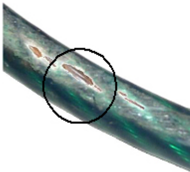
Figure 5. Damaged plastic coated wire rope.
